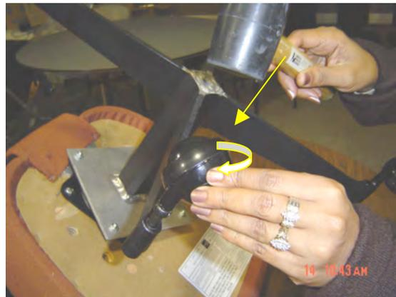
Align new caster and pin with the hole in the chair base. Using a rubber mallet, tap downwards on the caster. After each hit, rotate the caster so that you do not flatten the caster ball. Continue until the caster is fully seated into the hole in the chair base.
