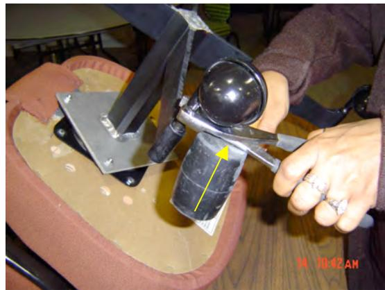
Grip the caster pin, near the base, with channel lock or vise grip pliers. Using a rubber mallet, tap in an upward motion until the caster and pin are removed.
